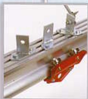
AT03 SINGLE BOLT HANGER Maximum capacity 250kg. Mounts parallel, 90 degree and 45 degree for suspension and bracing.
