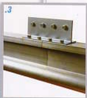
Completed joint accurately aligned for smooth running.
