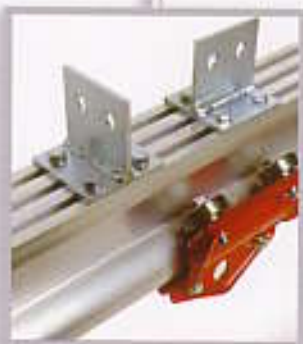
AT02 TWO BOLT HANGER Maximum capacity 500kg. Mounts parallel and 90 degree for suspension and bracing.
